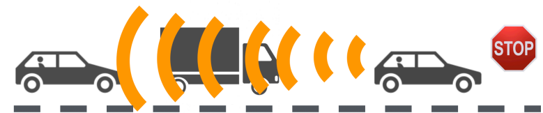
Vehicle-to-Vehicle (V2V) forward collision alerts based on network connectivity
